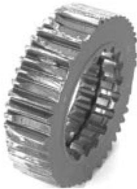
*Replace lube and bearings when damage to gearing appears similar to or worse than damage on this gear. Replacement is required due to fine particle contamination.*
