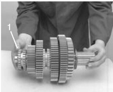
2. Place the mainshaft in a vertical position, pilot end down.
