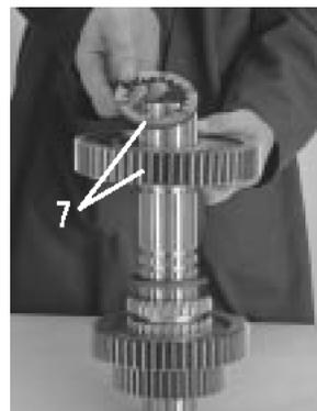
8. Remove the offset washer and sliding clutch.
