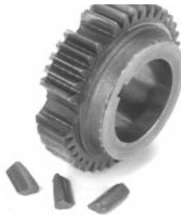
*Re-use lube and bearings when damage to gearing appears similar to damage on this gear.*
